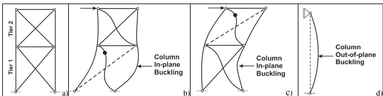
Fig. 3. a) Two-tiered steel braced frame; b) Column in-plane buckling following brace yielding in Tier 1; c) Column in-plane buckling following brace yielding in Tier 2; d) Column out-of-plane buckling.
