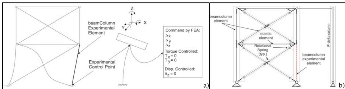
*Fig. 4.* a) Experimental control point assigned to the numerical substructure and experimental substructure; b) Hybrid numerical model of two-tiered concentrically braced frame.
