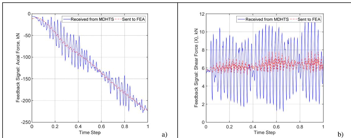
*Fig. 5.* Feedback signals: a) Axial force during gravity analysis; and b) Shear force during dynamic analysis.
