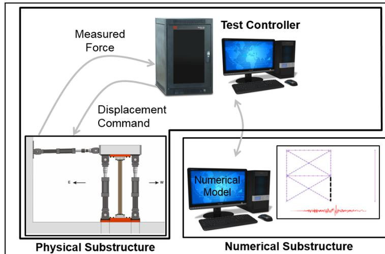
Fig. 2. Hybrid simulation loop.
