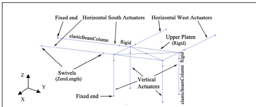
*Fig. 6.* *OpenSees* model of the MDHTS used to remove friction forces developing in the physical testing system.
