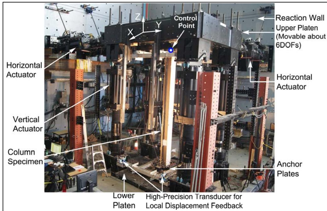
Fig. 1. I-shaped column specimen in the Multi-Directional Hybrid Testing System.
