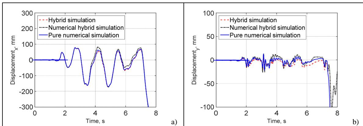
Fig. 8. Comparison of the displacements along X (in-plane) and Y (out-of-plane) axes at the top of the first-tier column segment as obtained from the pure numerical, hybrid simulations and hybrid testing.
