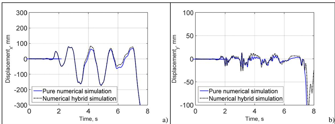
Fig. 7. Comparison of the displacements along X (in-plane) and Y (out-of-plane) axes at the top of the first-tier column segment as predicted by the pure numerical and numerical hybrid simulations.
