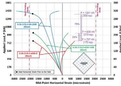
Figure 4: Applied load vs. horizontal steel strain with CFRP strands at an angle of:
