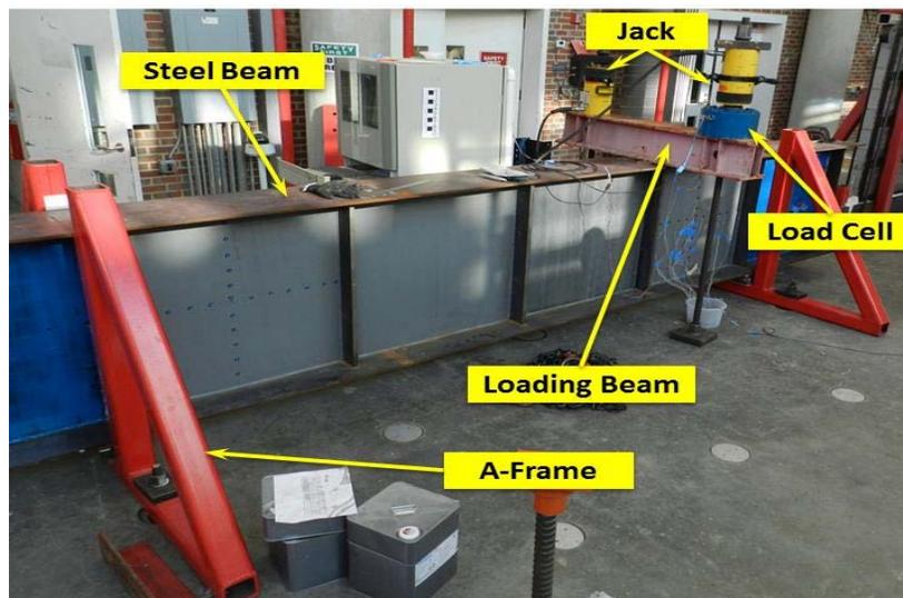
Figure 7: Steel girder test setup
