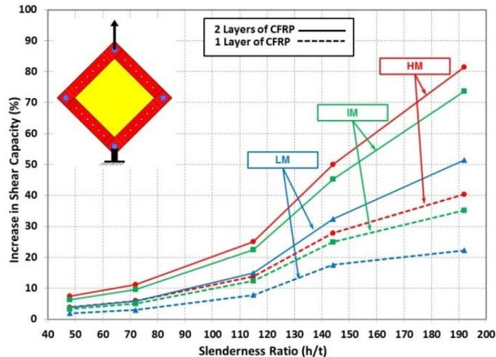
Figure 6: Percentage increase in shear capacity vs slenderness ratio of plates strengthened with one and two layers of HM, IM, and LM CFRP strands oriented 45° relative to the vertical tensile load
