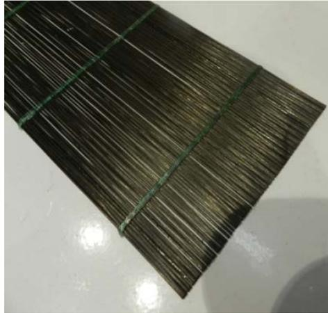
Figure 1: Proposed small-diameter CFRP strands
