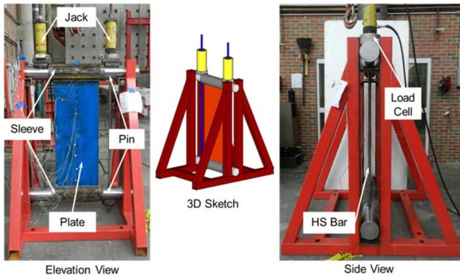
Figure 2: Test setup for uniaxial compression testing of plates
