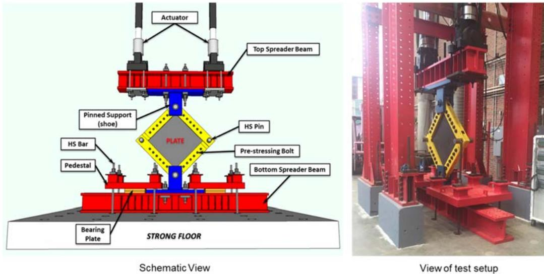
Figure 3: Pure shear test setup
