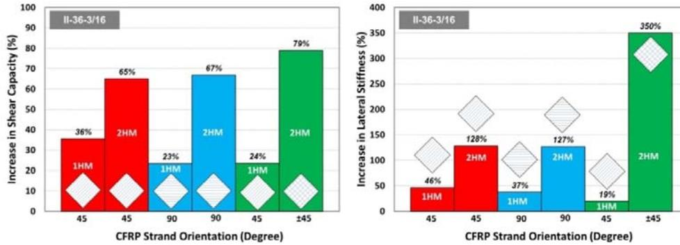
Figure 5: Shear capacity and lateral stiffness percentage increase of plates strengthened with one and two layers of HM CFRP strands
