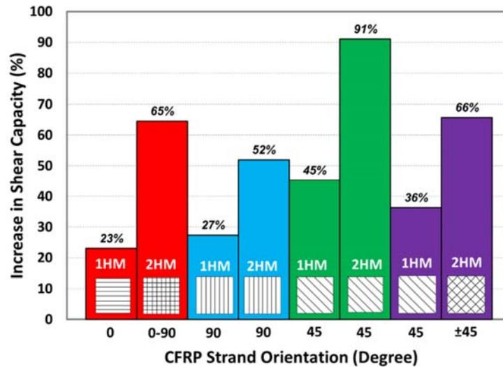
Figure 8: Shear capacity percentage increase of steel web panel strengthened with one and two layers of HM CFRP
